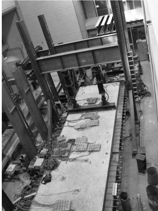
Figure 8 Laboratory bridge specimen during spreader beam test of Span 1
